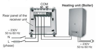
230 V mains voltage should be supplied to the receiver unit. We recommend using a fixed cable instead of a fork type connection for mains connection to avoid any unintentional de-energization of the device. We propose to connect the neutral wire of the network to point  ${\bf N}$ , while the phase conductor to point  ${\bf L}$ . We propose to interpose a switch so that the receiver unit can be de-energized if required.
